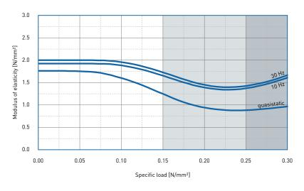
Dynamic test: sinusoidal excitation with an oscillating range of  $\pm$  0.11 mm at 10 Hz and  $\pm$  0.04 mm at 30 Hz
