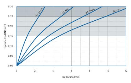
Recording of the 3rd loading; testing between steel plates at room temperature measured with a deflection rate of 1% of the thickness per second Form factor q=3
