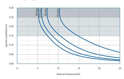
Natural frequency of a single-degree-of-freedom system consisting of a fixed mass and an elastic bearing consisting of PURASYS **vibra**dyn S 150 on a stiff subgrade.
